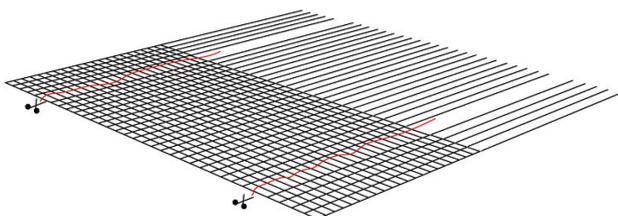
Fig. 1. Selvage formation in shuttle-less weaving machines.
