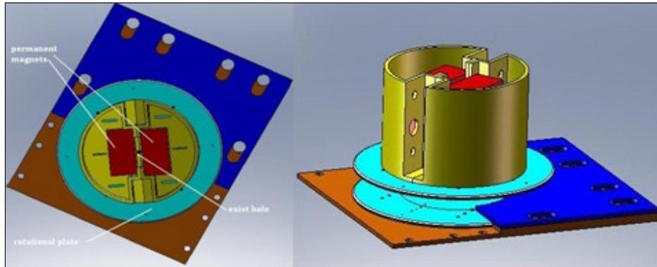
Figure 1: Unit designed for interlacing metallic filament
