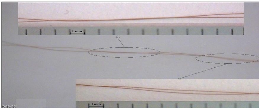
Figure 9: Two metallic filaments interlaced by the proposed method.
