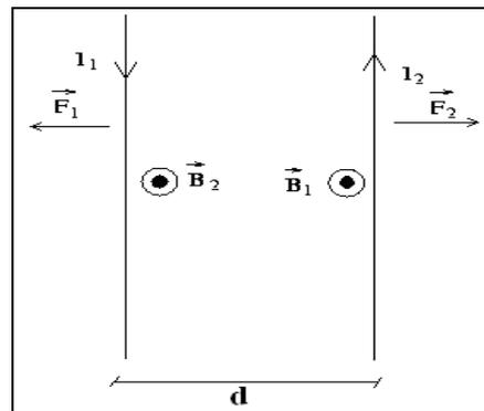
Figure 4: Force between two straight parallel conductive filaments
