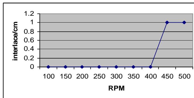
Figure 10: The effect of rotational speed of magnetic field on the number of interlaces per centimeter
