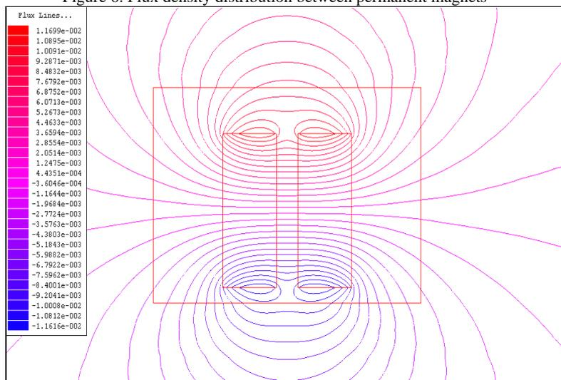
Figure 7: Flux distribution between permanent magnets
