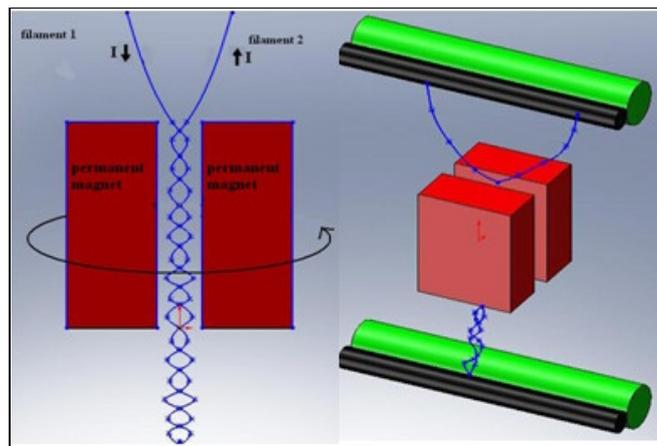
Figure 2: Schematic of interlacing zone
