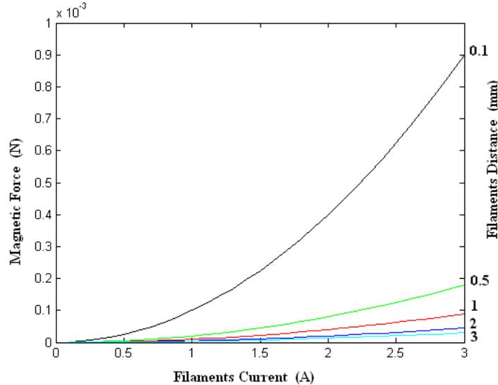
Figure 5: Magnetic force between two current-carrying conductive filaments
