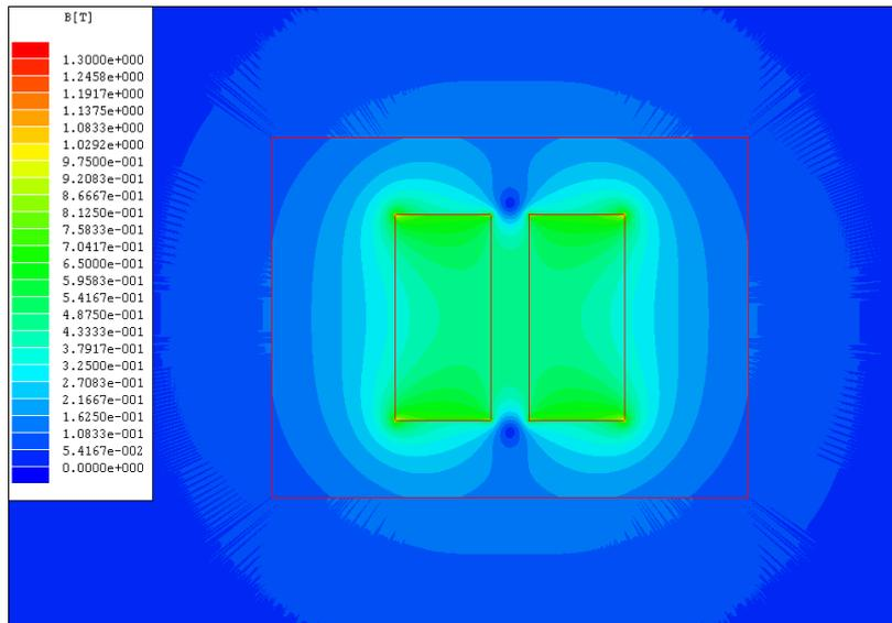
Figure 6: Flux density distribution between permanent magnets
