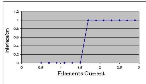
Figure 11: Effect of filaments currents on the number of interlaces per centimeter
